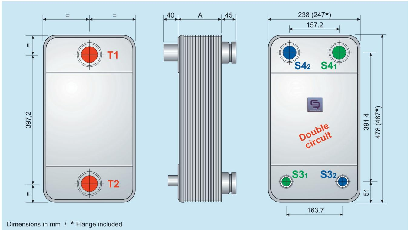
With the AC130 Alfa Laval has concentrated on reducing the dimensions to provide customers with a more compact heat exchanger. One advantage is immediately apparent: less room needed in the system. This is sometimes an advantage that is underestimated. Reduced space means not only more available room for other equipment, but also less obstruction to the air flow in many air units and a lighter weight to handle in the assembly line.
